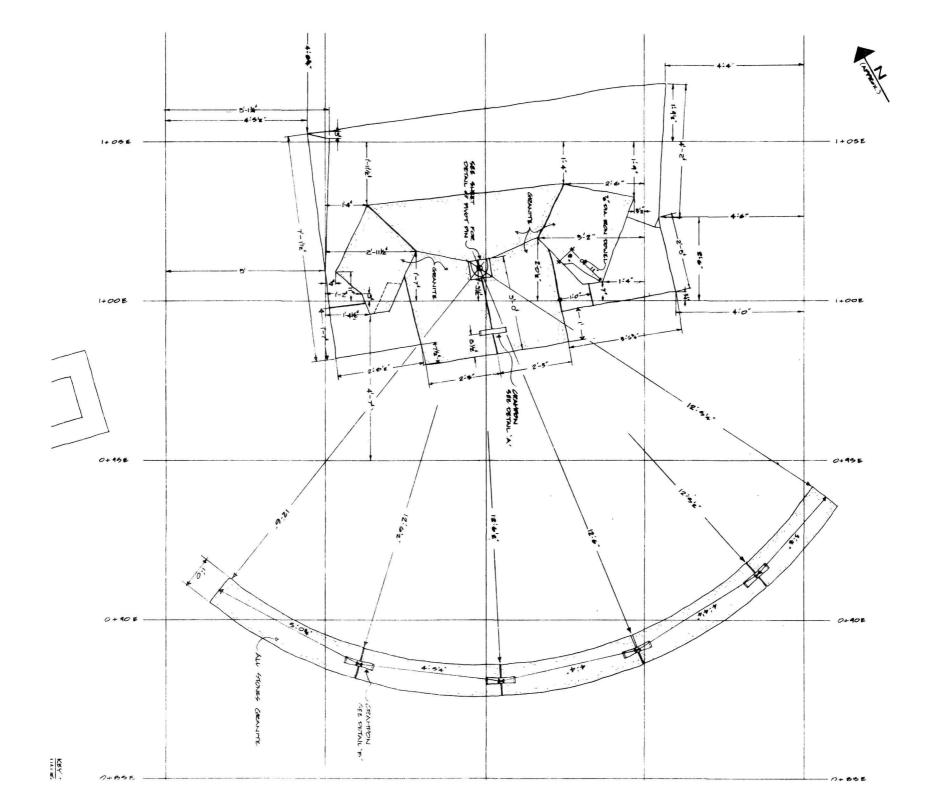
19 Preliminary field measurements on the complete emplacement on the right face of the northwest demi-bastion.
